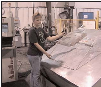
A K & S employee removes a wire frame from a state-of-the-art CNC wire forming machine.
